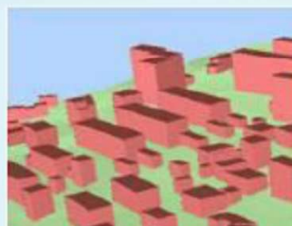
LoD1 Block models with no roof structures
