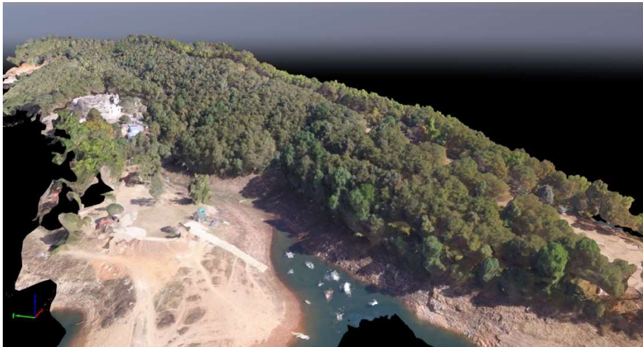
Full 3D Textured Model of Nehru Park, Umiam (made from 580 UAV Images)
